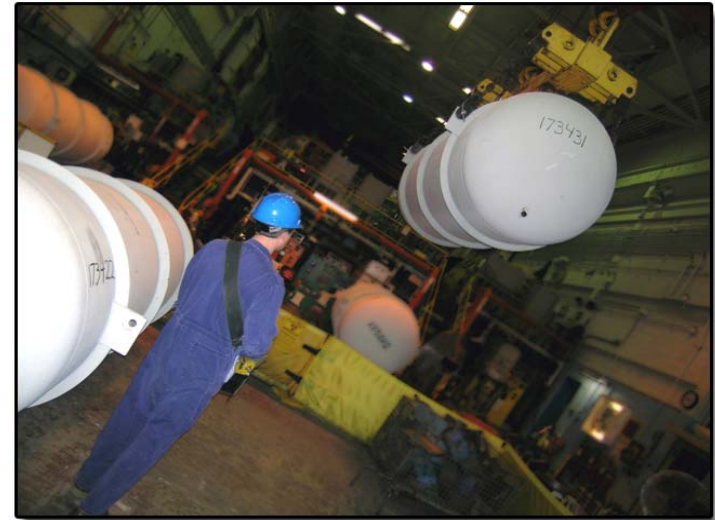
Uranium material handler uses radio-controlled overhead crane to place empty cylinder on autoclave used in Tc-99 removal. Process flows uranium through a trapping device to remove contaminants.
